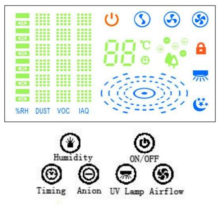
All buttons listed below from the left to the right are: First line: Humidity, ON/OFF; Second line: Timing, Anion, UV Lamp, Airflow
